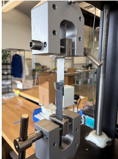
Figure 17. The prepared specimen is mounted to the jaws of the UTM instrument.
