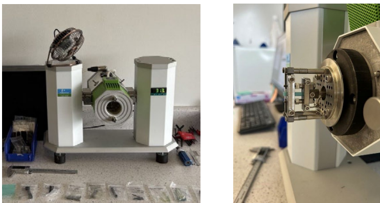
Figure 12. Perkin Elmer DMA 800 instrument (Left). The prepared sample shown above was loaded with a DMA instrument for testing (Right).
