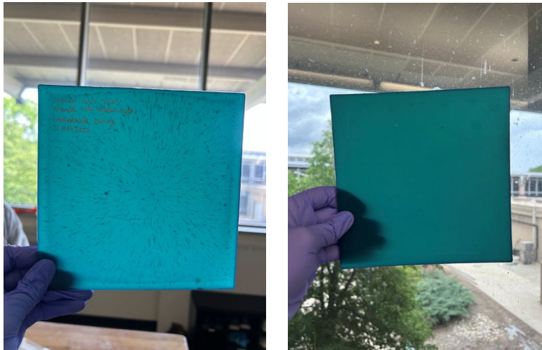
Figure 3. Initial injection mold panels showed air bubbles (Left). Air-free panels (Right).
