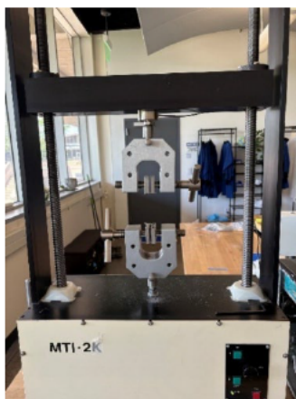
Figure 8. Universal testing machine with fixed and movable grips for holding the specimen.
