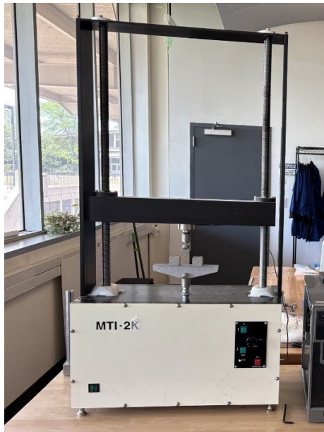
Figure 5. Universal testing machine (UTM) with the attached fixture to measure flexural properties of the specimens.
