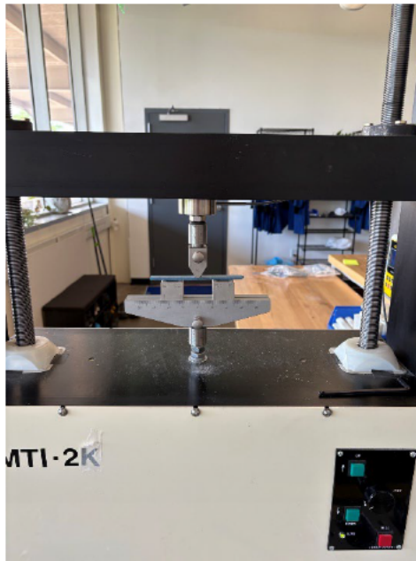
Figure 7. UTM with the attached fixture to measure flexural properties of the specimen. The waterjet cut specimen is centered on the support.
