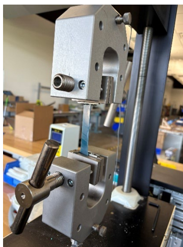
Figure 10. The close view of the UTM grips with the loaded specimen.
